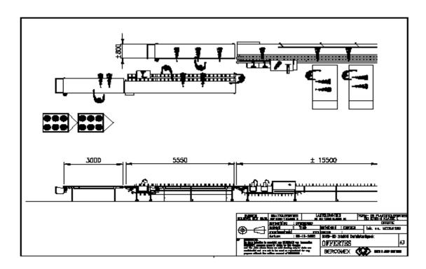
Flower processing line with a special packing section for roses (card board packaging). This packing line is designed to wrap SKF card board around the heads of a bunch of roses. The first person puts the SKF in the line, a second person puts a bunch on the card board while a third person closes the card board after which a binder automatically binds the bunch. Optional to bind twice, or extend the line to also put sleeve.
