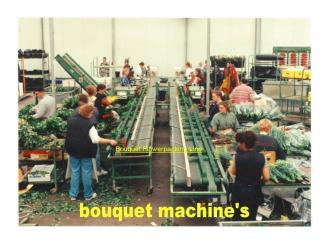
The capacity of the line is 750-3600 bunches per hour.
