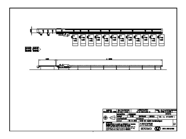
The Bercomex flower processing lines (also called bunching line) are used in over 90% of all European bouquet makers. Bunches are configured on the line or hand made on the workstations (the tables in the drawing) and placed on a conveyor belt. This belt takes the bunches through a processing unit, which may contain a saw, defoliator(s) and binder(s). After that a sleeving section may be included, optionally with flower food sachet binders and tapers.
